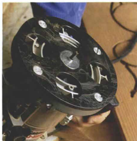
Making the brackets. Over a hundred pieces went into the brackets and modillions, making their fabrication perfect for template routing. In the photo to die right, the author routs the profile of an outer lamination. The next pass, with a \frac{1}{8} -in. bit and collet (above) will mill the fretwork pattern in its face.
